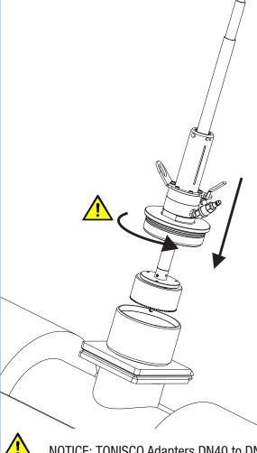
NOTICE: TONISCO Adapters DN40 to DN 125 are equiped with a right side thread while the sizes DN 150 and DN 200 equipped with left side threads.
