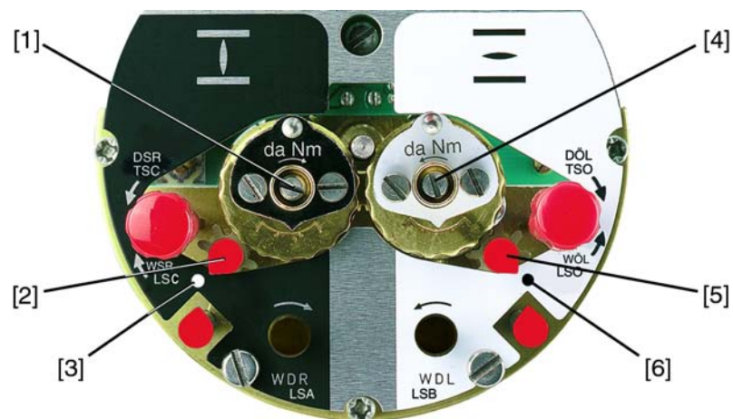
Figure 27: Setting elements for limit switching
