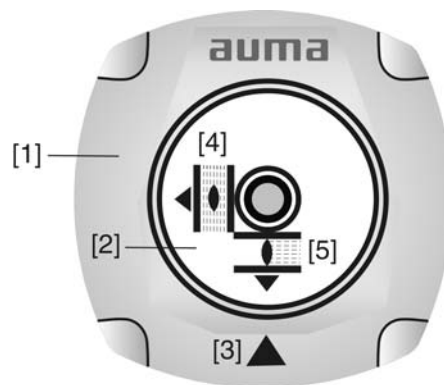
Figure 24: Mechanical position indicator
